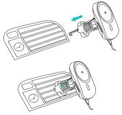
Fasten the air vent hook onto the air vent grille. Turn the lock to secure the hook in place.
