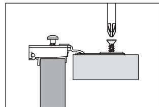
To hang the door to the cabinet, first align the door on the cabinet with the hinge arms on the edge of the face frame.
