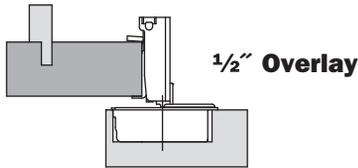
To install the hinge cup, drill a 1-3/8" hole (35 mm), 1/2" (12 mm) deep at a position of 3/32" (2.5 mm) from the edge of the door. Secure to the door using two #6 x 5/8" wood screws.
