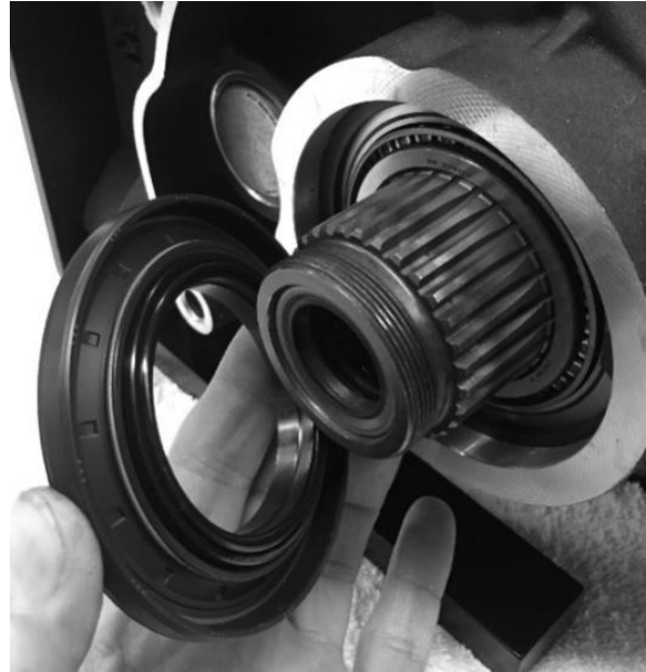
FIGURE 18 | INSTALLING THE PULLEY SPACER AND THE MAIN DRIVE GEAR SEAL
