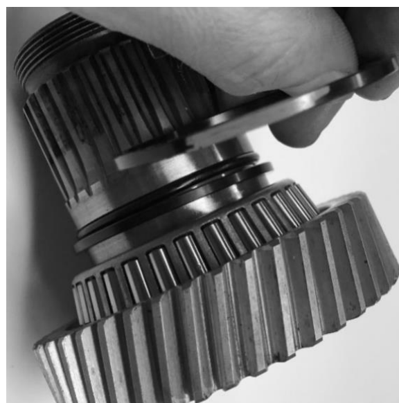
FIGURE 14 | MAIN DRIVE GEAR WITH PRE-INSTALLED SPACER AND ONE OF THE EXTRAS; LUBE O-RING
