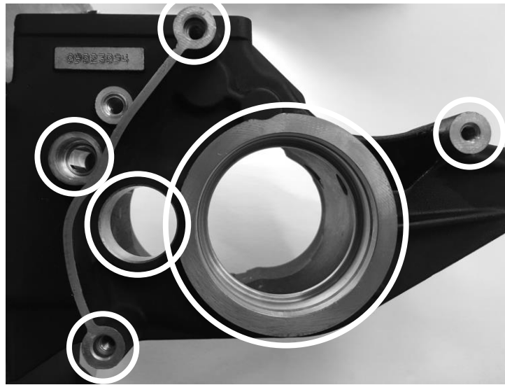
FIGURE 3 | SURGICALLY CLEAN THE LEFT SIDE OF THE TRANSMISSION CASE IN THE AREAS INDICATED ABOVE
