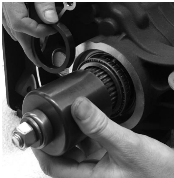
FIGURE 15 | IF USING H-D TOOLING, THE INCLUDED PULLEY SPACER IS NEEDED TO EXTEND THE LENGTH OF THE INSTALLATION CUP
