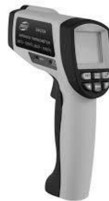
FIGURE 9 | USE AN INFRARED THERMOMETER TO VERIFY THAT THE CASE IS HEATED TO AT LEAST 200° F
