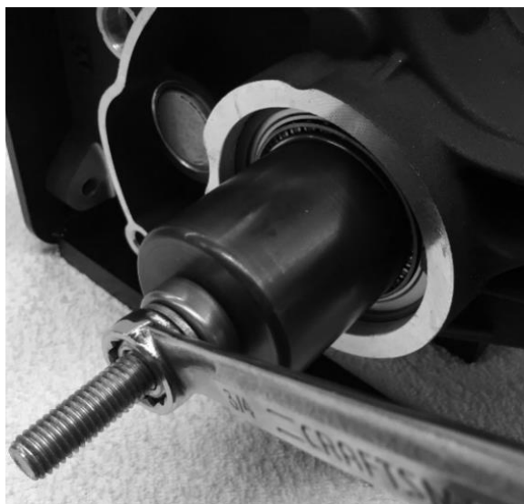
FIGURE 16 | INSTALLING THE MAIN DRIVE GEAR
