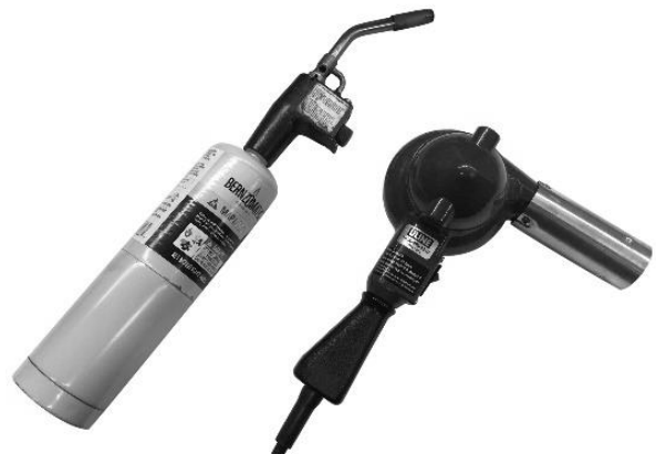
FIGURE 8 | USE MAP/PROPANE GAS OR A HEAT GUN TO HEAT THE CASE
