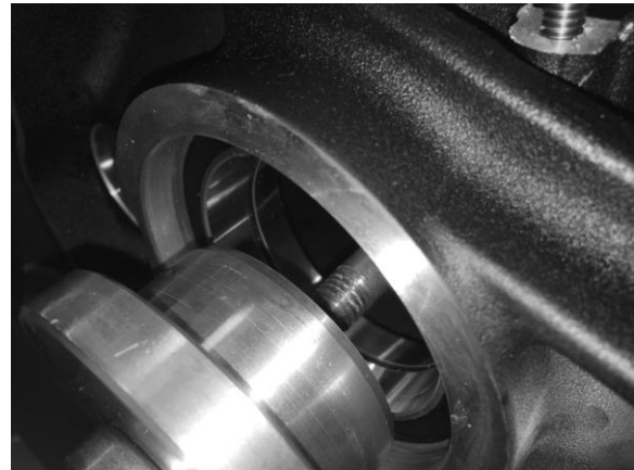
FIGURE 11 | TAPERED BEARING ADAPTER VISUAL INSPECTION
