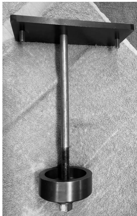
FIGURE 10 | TOOL SETUP FOR INSTALLING THE MAIN DRIVE GEAR BEARING
