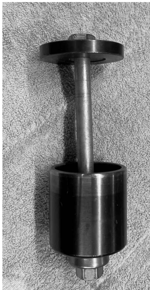
FIGURE 12 | TOOL SETUP FOR INSTALLING THE MAIN DRIVE GEAR
