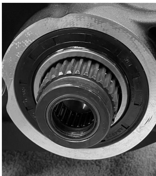
FIGURE 13 | MAIN DRIVE GEAR SEAL INSTALLED FLUSH WITH CASE
