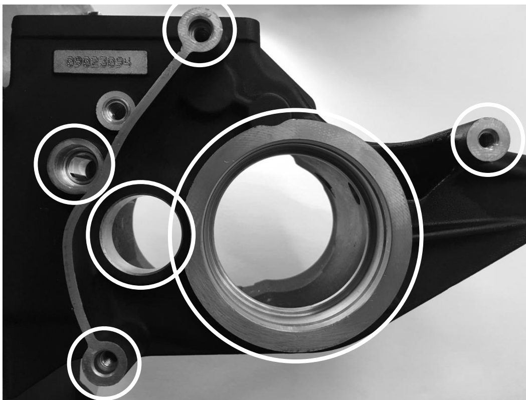
FIGURE 9 | SURGICALLY CLEAN THE LEFT SIDE OF THE TRANSMISSION CASE IN THE AREAS INDICATED ABOVE
