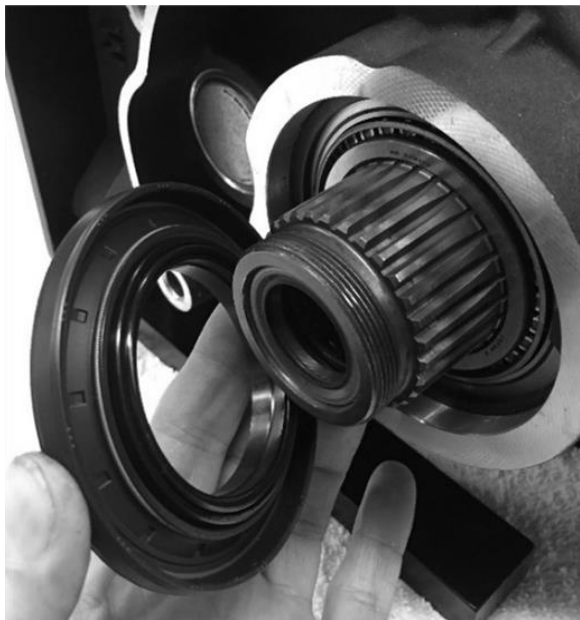
FIGURE 24 | INSTALLING THE PULLEY SPACER AND THE MAIN DRIVE GEAR SEAL
