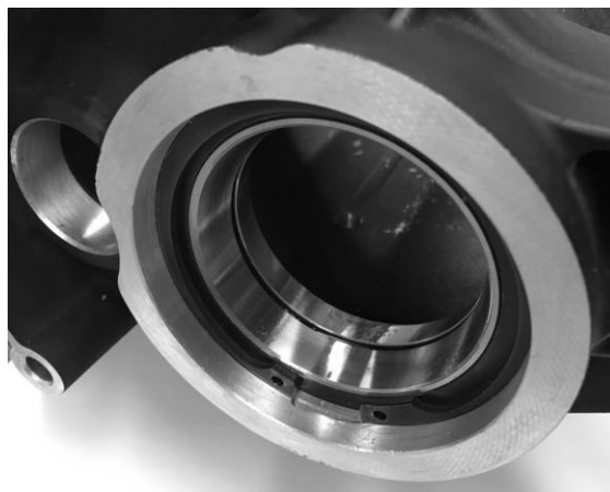
FIGURE 19 | LIGHTLY OIL BEARING RACES BEFORE INSTALLING THE MAIN DRIVE GEAR
