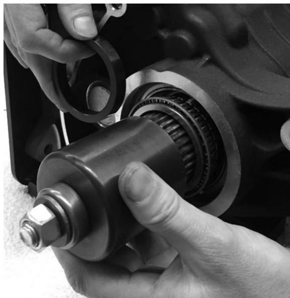
FIGURE 21 | IF USING H-D TOOLING, THE PULLEY SPACER IS NEEDED TO EXTEND THE LENGTH OF THE INSTALLATION CUP
