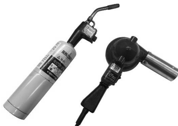
FIGURE 14 | USE MAP/PROPANE GAS OR A HEAT GUN TO HEAT THE CASE
