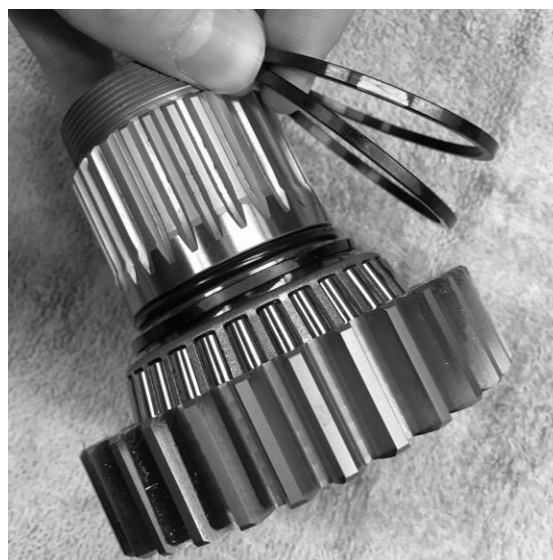
FIGURE 20 | MAIN DRIVE GEAR WITH PRE-INSTALLED SPACER AND TWO OF FIVE EXTRA SPACERS SHOWN; LUBE O-RING EACH TIME SPACER IS CHANGED
