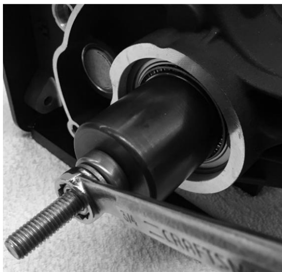
FIGURE 22 | INSTALLING THE MAIN DRIVE GEAR
