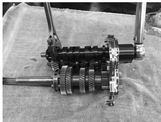
**FIGURE 25 | TORQUE SHIFT DRUM TO 20-25 FT-LBS**
