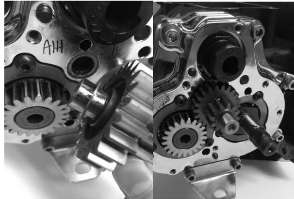
**FIGURE 28 | INSTALLING THE THRUST WASHER AND SPLIT IDLER GEAR**
