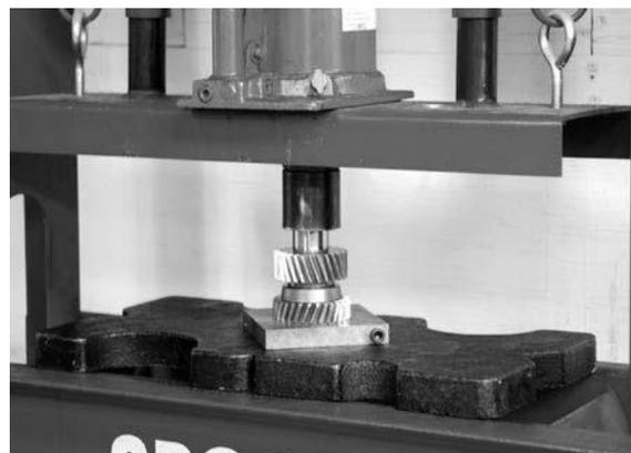
FIGURE 15 | PRESSING 5<sup>TH</sup> COUNTER GEAR ONTO THE F6R COUNTERSHAFT
