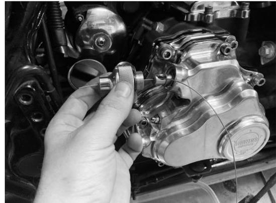
FIGURE 43 | CABLE IN PLUNGER AND CAP ASSEMBLY
