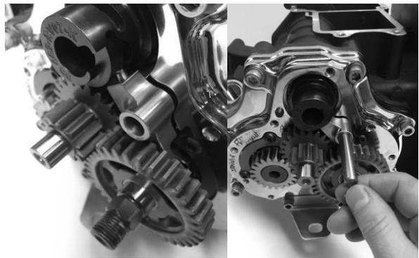
**FIGURE 30 | INSTALLING THE REVERSE SHIFT FORK AND FORK ROD**
