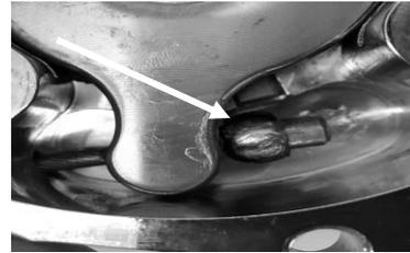
FIGURE 33 | INSTALLING CLUTCH CABLE FERRULE
