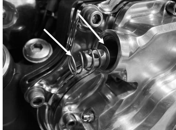
FIGURE 42 | WASHER AND SAFETY SPRING ON PLUNGER
