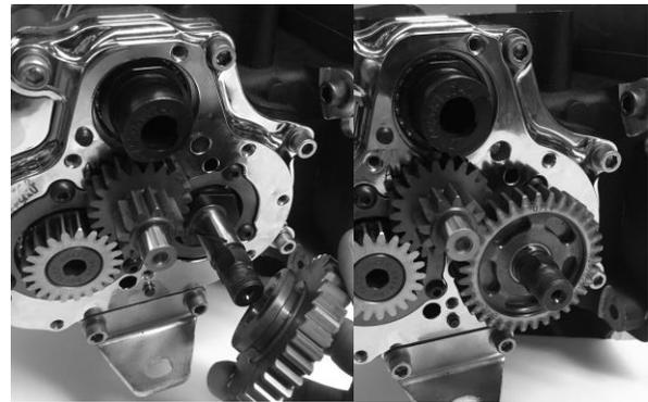
**FIGURE 29 | INSTALLING THE REVERSE SLIDER GEAR ONTO THE COUNTERSHAFT**
