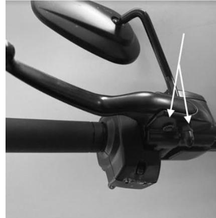
**FIGURE 48 | SAFETY LEVER MOUNT POSITION**
