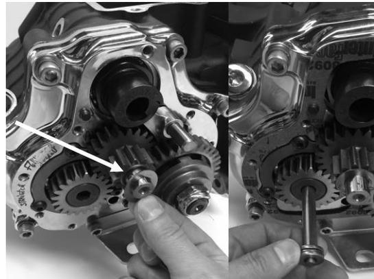
FIGURE 40 | THRUST WASHER, RELEASE AND ACTUATOR ROD INSTALLATION
