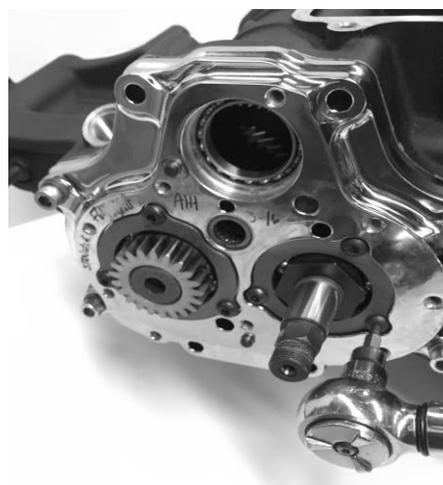
**FIGURE 22 | INSTALL RETAINER PLATE AND TORQUE TO 130 IN-LBS**
