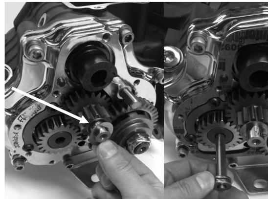
FIGURE 37 | THRUST WASHER, RELEASE AND ACTUATOR ROD INSTALLATION
