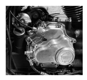
FIGURE 44 | CABLE HOUSING INSTALLED TO THREADED CAP
