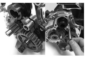
FIGURE 30 | INSTALLING THE REVERSE SHIFT FORK AND FORK ROD
