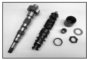
F6R Countershaft with Spacer & Retainer Shift Drum with Drum Nut Socket, Shift Drum Mainshaft Retainer
