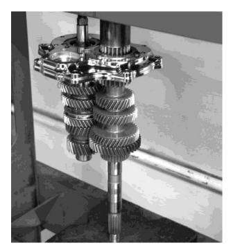
FIGURE 18 | ALIGN THE MAINSHAFT WITH THE COUNTERSHAFT AND START THE END OF THE SHAFT INTO THE BEARING. POSTION THE SHAFT ON THE PRESS.
