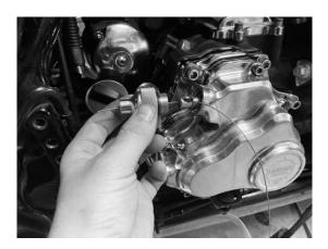
FIGURE 43 | CABLE IN PLUNGER AND CAP ASSEMBLY
