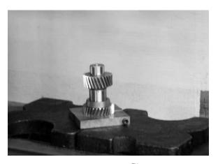
FIGURE 14 | PRESSING 5<sup>TH</sup> COUNTER GEAR ONTO THE F6R COUNTERSHAFT
