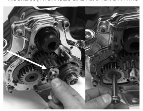
FIGURE 37 | THRUST WASHER, RELEASE AND ACTUATOR ROD INSTALLATION
