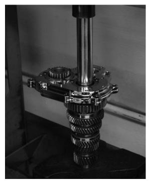
FIGURE 17 | PRESSING ON THE INNER RACE INSTALLATION TOOL
