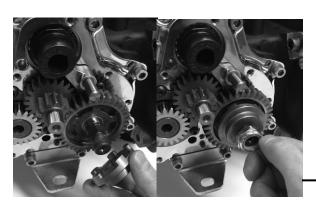
FIGURE 31 | INSTALLING THE REVERSE SHIFT DOG CLUTCH AND NYLOCK NUT
