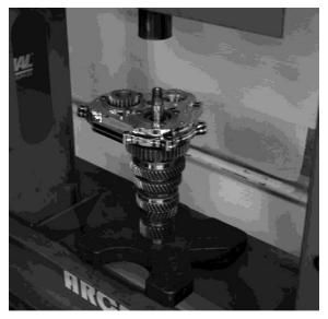
FIGURE 16 | ALIGNING DOOR TO COUNTERSHAFT
