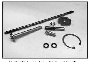
Center Release Rod – Kit Type Specific Auxiliary Rod Adjuster Plate, Screw, Nut and Retaining Snap Ring – Kit Type Specific Banjo Bolt with Seals
