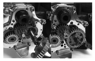
FIGURE 29 | INSTALLING THE REVERSE SLIDER GEAR ONTO THE COUNTERSHAFT
