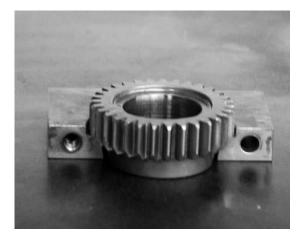
FIGURE 12 | SPLIT BEARING PRESS TOOL HALF SHOWN WRAPPING  $5^{\rm TH}$  COUNTER GEAR
