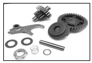
Reverse Shift Fork and Rod Reverse Idler Gear with Thrust Washers Safety Plunger Washer and Spring Reverse Gear Reverse Shift Dog with Nylock Nut
