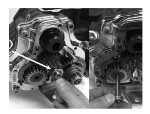
FIGURE 40 | THRUST WASHER, RELEASE AND ACTUATOR ROD INSTALLATION
