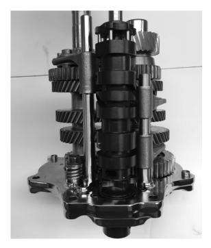
FIGURE 26 | SHIFT FORK AND FORK ROD INSTALLATION
