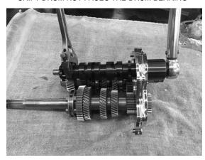
FIGURE 25 | TORQUE SHIFT DRUM TO 20-25 FT-LBS
