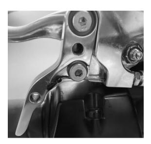
FIGURE 51 SAFETY CABLE TERMINATION AND THUMB LEVER
