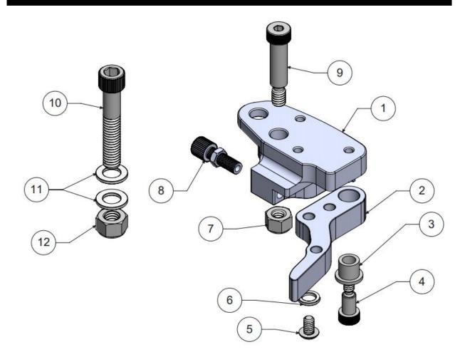
FIGURE 6 | SAFETY LEVER AND MOUNT
