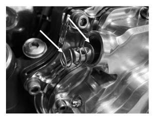
FIGURE 42 | WASHER AND SAFETY SPRING ON PLUNGER
