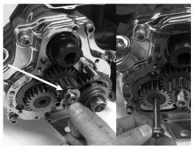
FIGURE 34 | THRUST WASHER, RELEASE AND ACTUATOR ROD INSTALLATION
