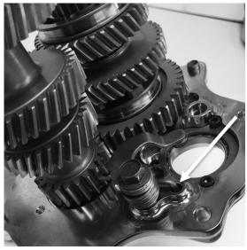
FIGURE 23 | INSTALLATION OF THE SHIFT DRUM DETENT LEVER
