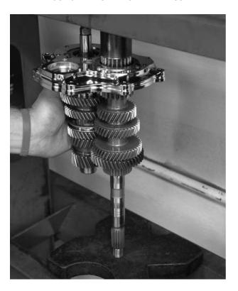
FIGURE 19 | WITH THE MAINSHAFT SQUARE TO THE PRESS, PRESS ON THE MAINSHAFT SIDE OF THE PINION GEAR UNTIL FULLY SEATED
