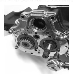
FIGURE 22 | INSTALL RETAINER PLATE AND TORQUE TO 130 IN-LBS
