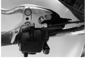
FIGURE 49 | SAFETY LEVER INSTALLED
