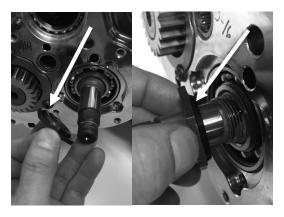
FIGURE 21 | INSTALL THE SNOUT OF THE COUNTERSHAFT BASE NUT FACING THE BEARING
