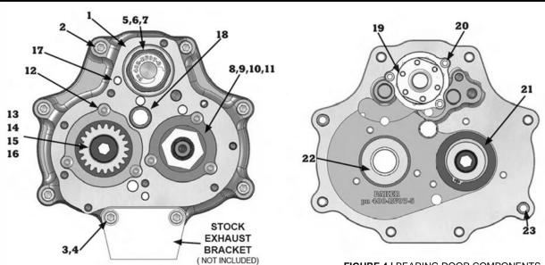
FIGURE 4 | BEARING DOOR COMPONENTS
