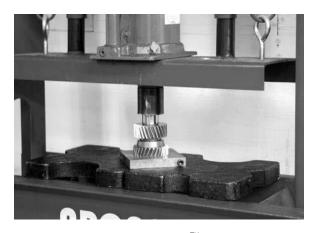
FIGURE 15 | PRESSING  $5^{TH}$  COUNTER GEAR ONTO THE F6R COUNTERSHAFT
