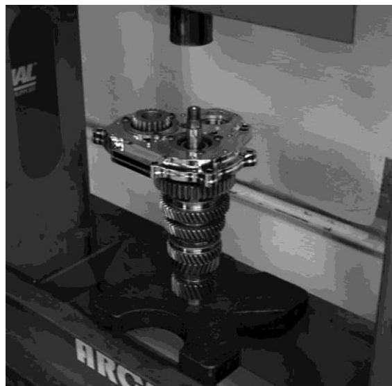
FIGURE 16 | ALIGNING DOOR TO COUNTERSHAFT
