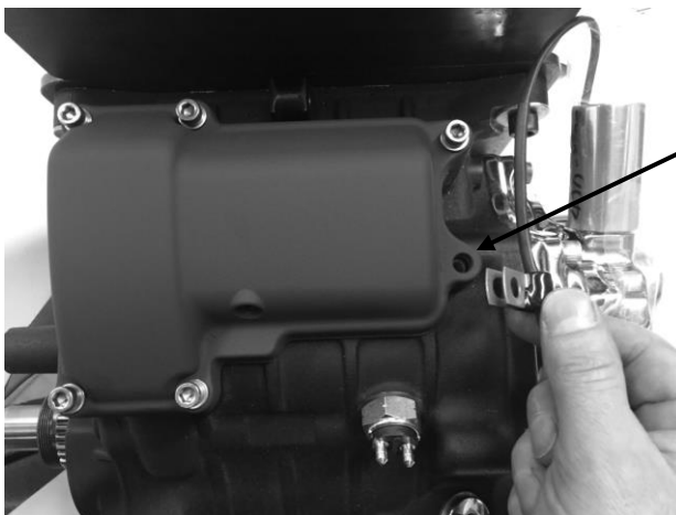
FIGURE 28 | SOLENOID WIRING CLAMP ON TOP COVER
