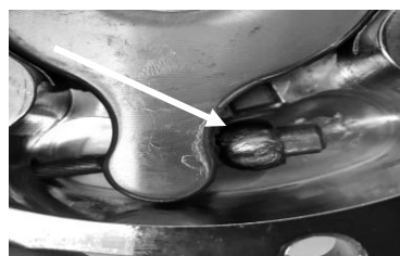
FIGURE 34 | INSTALLING CLUTCH CABLE FERRULE
