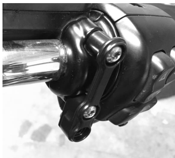
FIGURE 47 | SWITCH HOUSING PERCH CLAMP LOOSELY INSTALLED; NOT TORQUED
