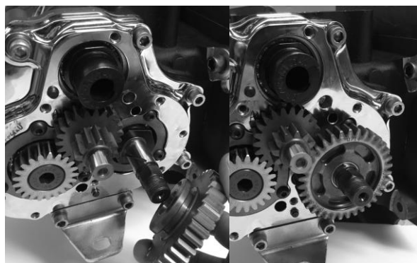
FIGURE 30 | INSTALLING THE REVERSE SLIDER GEAR ONTO THE COUNTERSHAFT
