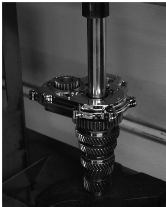
FIGURE 17 | PRESSING ON THE INNER RACE INSTALLATION TOOL
