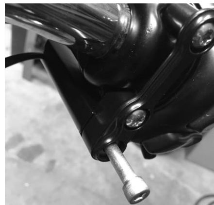
FIGURE 49 | INSTALLATION OF BRACKET ASSEMBLY WITH HARNESS
