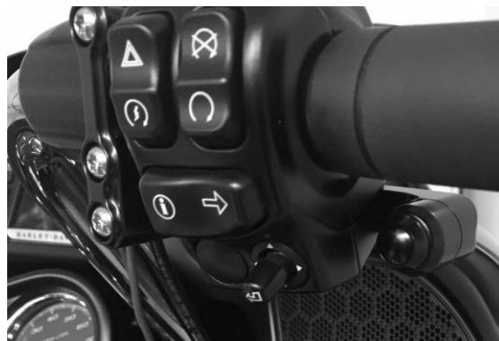
FIGURE 50 | F6R SWITCH HOUSING INSTALLED
