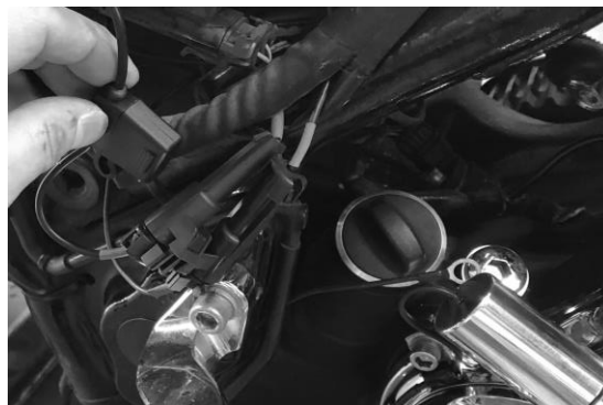
FIGURE 53 | CONNECTING THE SOLENOID WIRING HARNESS – RIGHT SIDE OF BIKE, TOURING MODEL SHOWN
