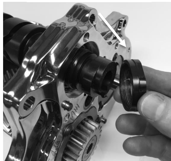
FIGURE 24 | ROUNDED END OF SPECIAL SHIFT DRUM NUT FACES THE DRUM BEARING
