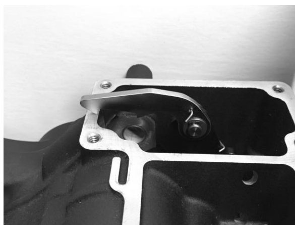
FIGURE 11 | LIFT THE PAWL ARM ONTO THE GASKET
