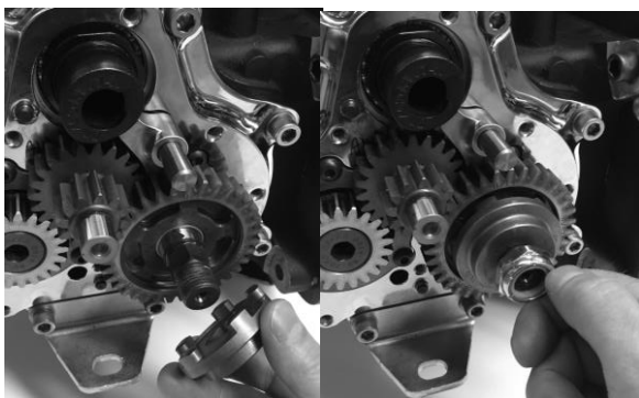
FIGURE 32 | INSTALLING THE REVERSE SHIFT DOG CLUTCH AND NYLOCK NUT
