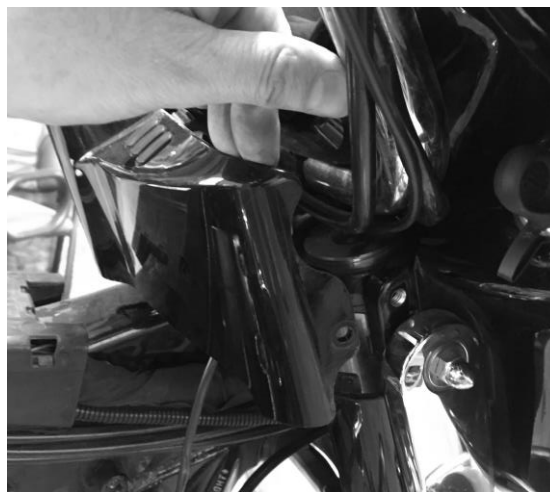
FIGURE 51 | PULL BACK THE DASH PANEL TO ROUTE WIRING BEHIND THE BARS
