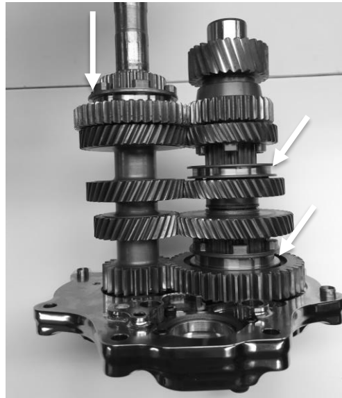
FIGURE 20 | LOCK THE GEARSET BY ENGAGING AT LEAST TWO OF THE SHIFT DOGS
