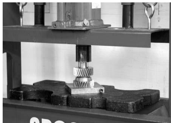
FIGURE 15 | PRESSING 5 TH COUNTER GEAR ONTO THE F6R COUNTERSHAFT
