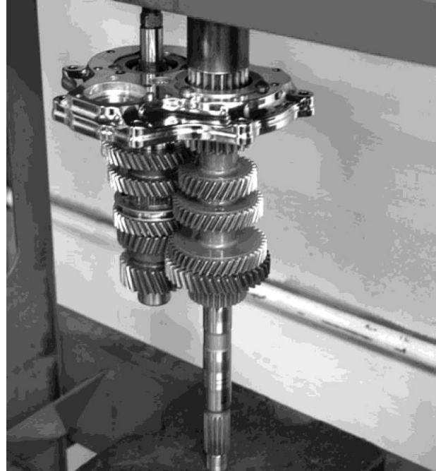
FIGURE 18 | ALIGN THE MAINSHAFT WITH THE COUNTERSHAFT AND START THE END OF THE SHAFT INTO THE BEARING. POSITION THE SHAFT ON THE PRESS.
