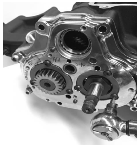
FIGURE 22 | INSTALL RETAINER PLATE AND TORQUE TO 130 IN-LBS
