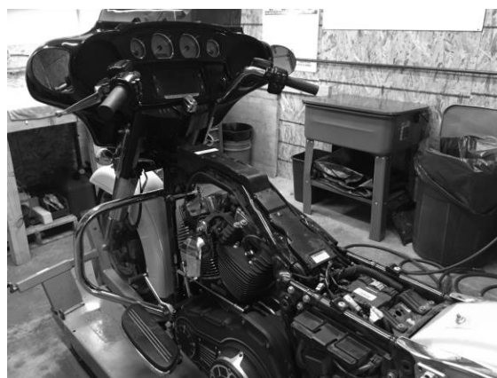
FIGURE 46 | TOURING MODEL WITH TANK REMOVED FOR WIRING
