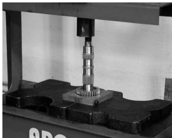
FIGURE 13 | PRESSING OFF 5 TH COUNTER GEAR FROM THE COUNTERSHAFT USING THE SPLIT BEARING TOOL
