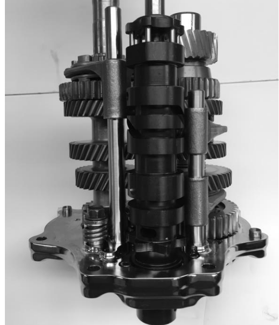
FIGURE 26 | SHIFT FORK AND FORK ROD INSTALLATION
