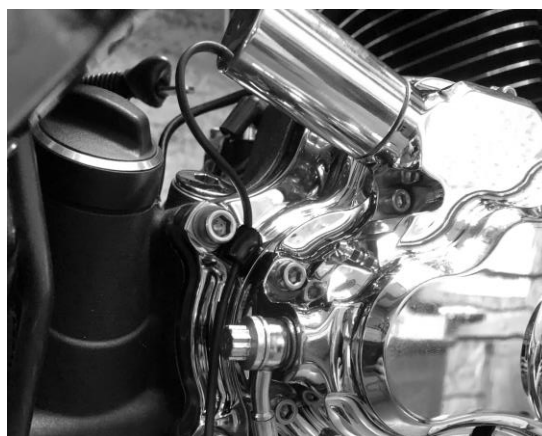
FIGURE 45 | REAR SOLENOID WIRE ROUTING – TOURING MODELS
