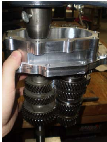
*Mainshaft and Countershaft Assembly Pressed In
