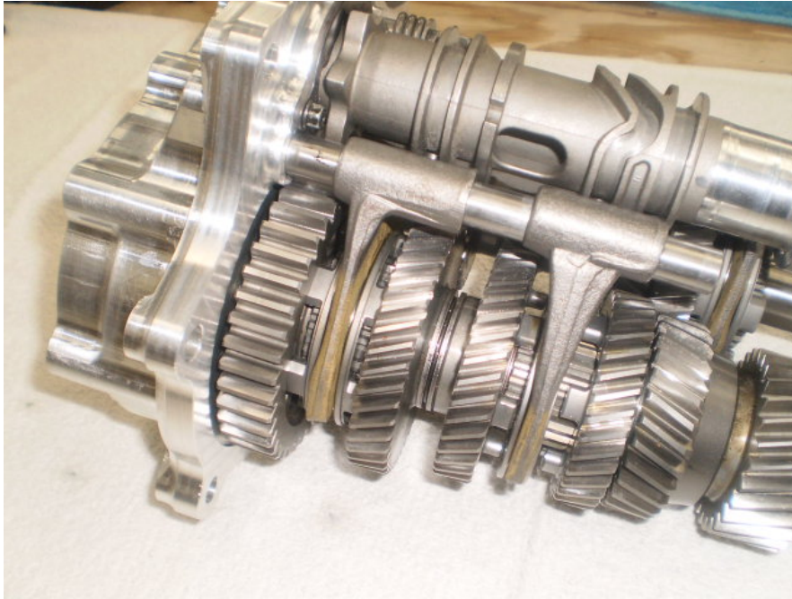
*Completed F6K bearing Door Assembly
