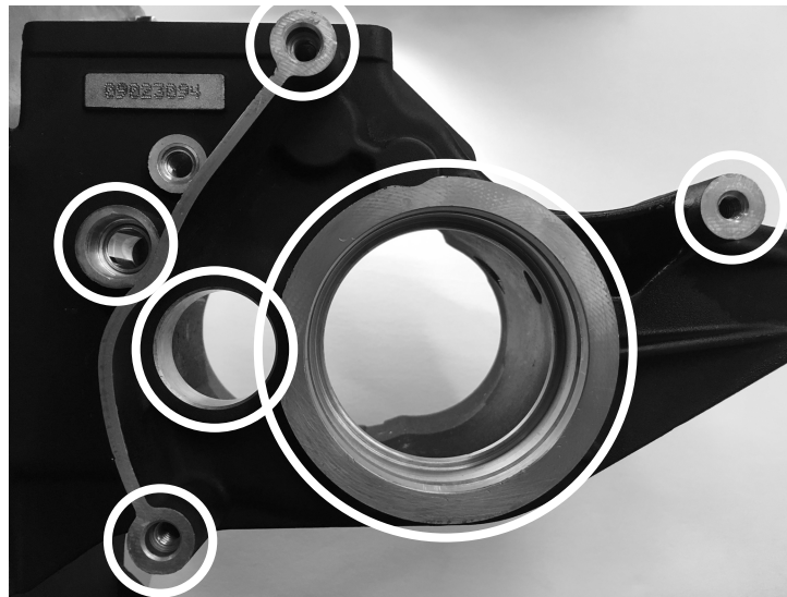
FIGURE 7 | SURGICALLY CLEAN THE LEFT SIDE OF THE TRANSMISSION CASE IN THE AREAS INDICATED ABOVE
