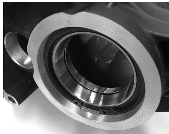
FIGURE 17 | LIGHTLY OIL BEARING RACES BEFORE INSTALLING THE MAIN DRIVE GEAR
