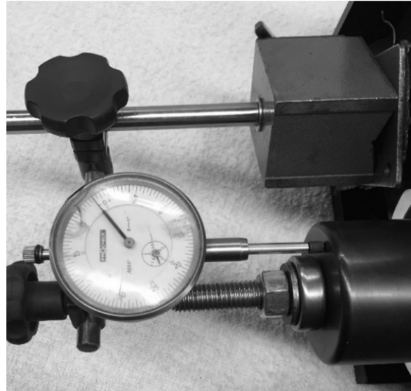
FIGURE 21 | CHECKING AXIAL END PLAY IN THE MAIN DRIVE GEAR TAPERED ROLLER BEARING
