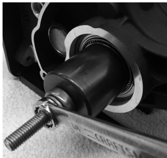
FIGURE 20 | INSTALLING THE MAIN DRIVE GEAR
