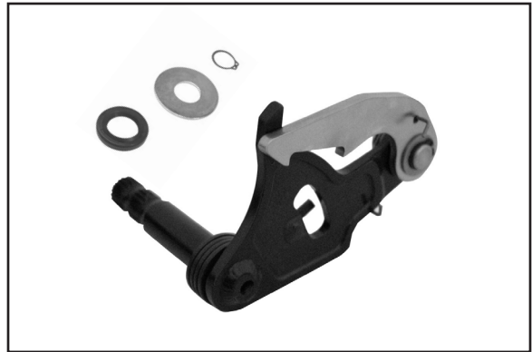
Shifter pawl, 555-07-A Shifter pawl washer, 6497HW-HD Shifter pawl retaining ring, 68010 Shifter pawl seal, 11000101
