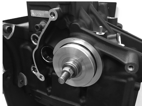
FIGURE 9 | TAPERED BEARING ADAPTER TOOL SETUP, LEFT SIDE VIEW
