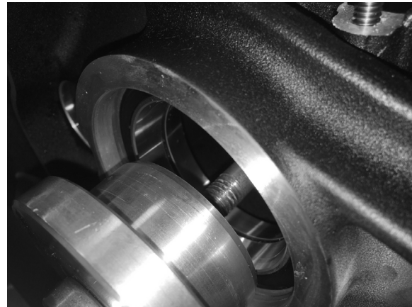
FIGURE 15 | TAPERED BEARING ADAPTER VISUAL INSPECTION
