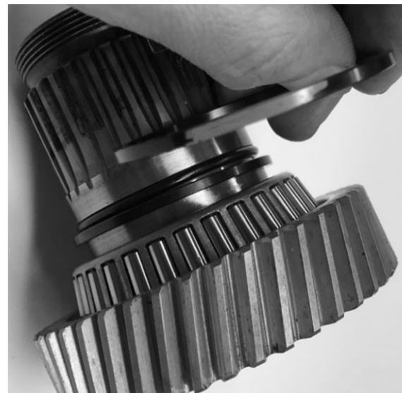
FIGURE 18 | MAIN DRIVE GEAR WITH PRE-INSTALLED SPACER AND ONE OF THE EXTRAS; LUBE O-RING
