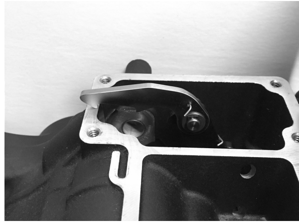
FIGURE 24 | LIFT THE PAWL ARM ONTO THE GASKET SURFACE UNTIL THE GEARSET IS INSTALLED AND THE BOLTS ARE TORQUED
