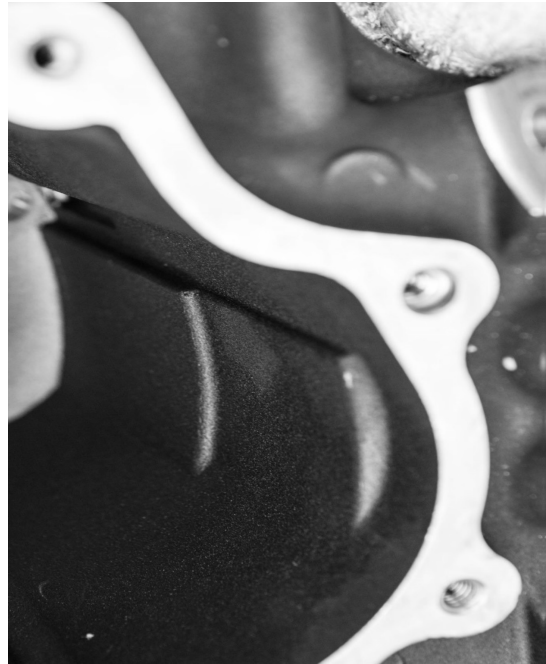
FIGURE 26 | INSIDE OF THE STOCK CASE; NO GEAR TO CASE INTERFERENCE SEEN ON THE INSIDE.
