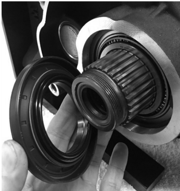
FIGURE 22 | INSTALLING THE PULLEY SPACER AND THE MAIN DRIVE GEAR SEAL
