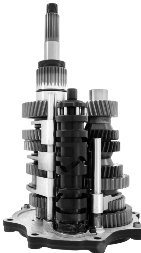
FIGURE 25 | DD7 GEARSET READY FOR INSTALLATION INTO THE CASE
