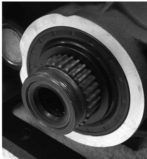
FIGURE 23 | MAIN DRIVE GEAR SEAL INSTALLED FLUSH WITH CASE
