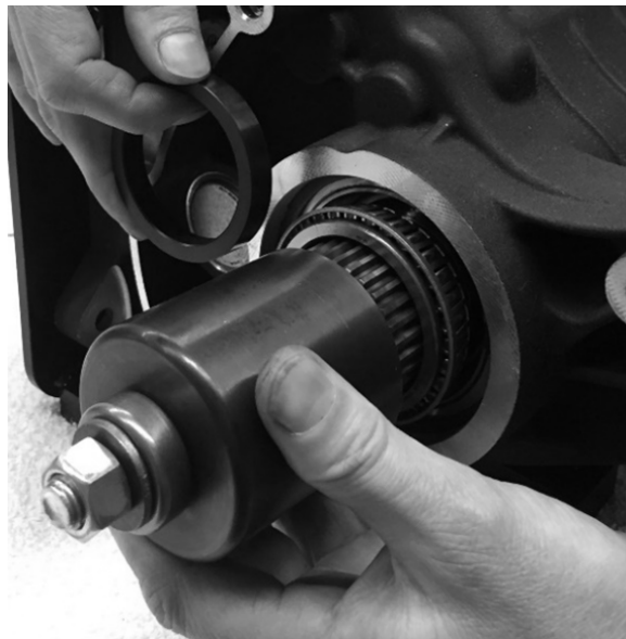
FIGURE 19 | IF USING H-D TOOLING, THE PULLEY SPACER IS NEEDED TO EXTEND THE LENGTH OF THE INSTALLATION CUP
