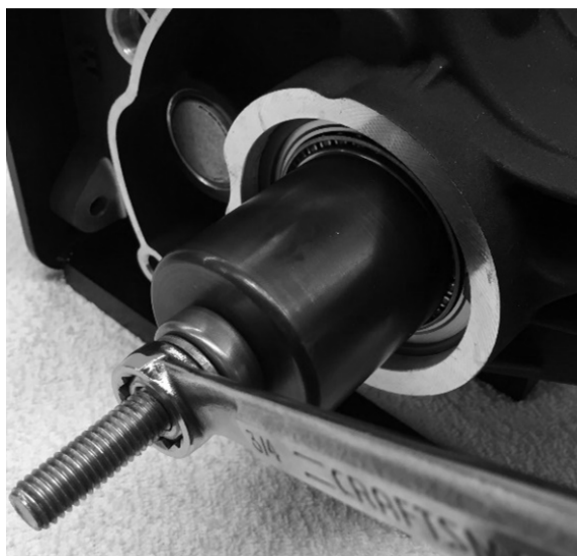
FIGURE 20 | INSTALLING THE MAIN DRIVE GEAR
