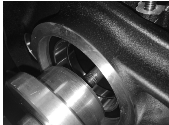
FIGURE 15 | TAPERED BEARING ADAPTER VISUAL INSPECTION
