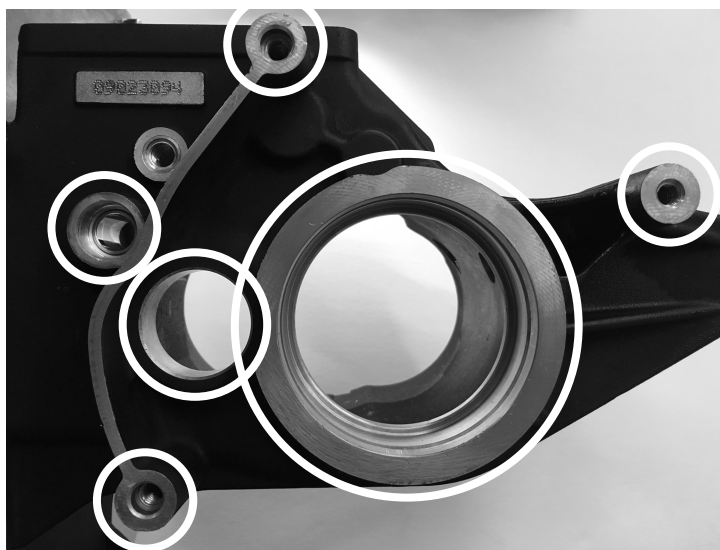
FIGURE 7 | SURGICALLY CLEAN THE LEFT SIDE OF THE TRANSMISSION CASE IN THE AREAS INDICATED ABOVE
