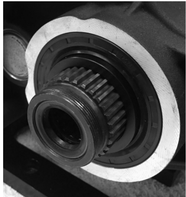
FIGURE 23 | MAIN DRIVE GEAR SEAL INSTALLED FLUSH WITH CASE
