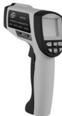
FIGURE 13 | USE AN INFRARED THERMOMETER TO VERIFY THAT THE CASE IS HEATED TO AT LEAST 200° F
