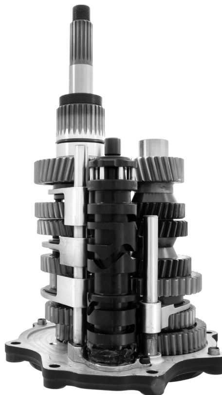
FIGURE 25 | DD7 GEARSET READY FOR INSTALLATION INTO THE CASE
