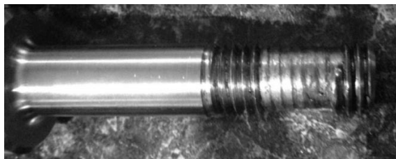
Figure 5, Destroyed Bolt Threads
