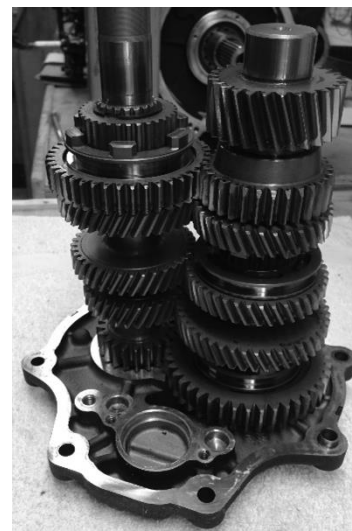
FIGURE 3 | STOCK SHIFT SYSTEM REMOVED
