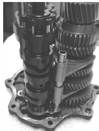
FIGURE 5 | NEW BAKER SHIFT SYSTEM INSTALLED
