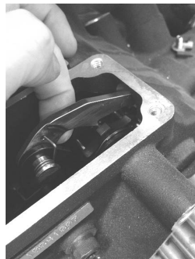
FIGURE 7 | LIFT PAWL ARM OVER SHIFT DRUM DURING INSTALLATION
