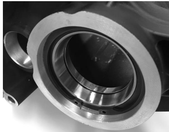
FIGURE 13 | LIGHTLY OIL BEARING RACES AFTER INSTALLING THE TAPERED BEARING ADAPTER
