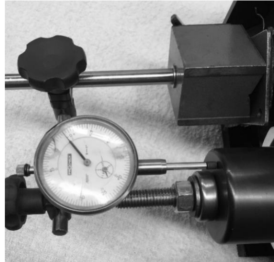
FIGURE 17 | CHECKING AXIAL END PLAY IN THE MAIN DRIVE GEAR TAPERED ROLLER BEARING
