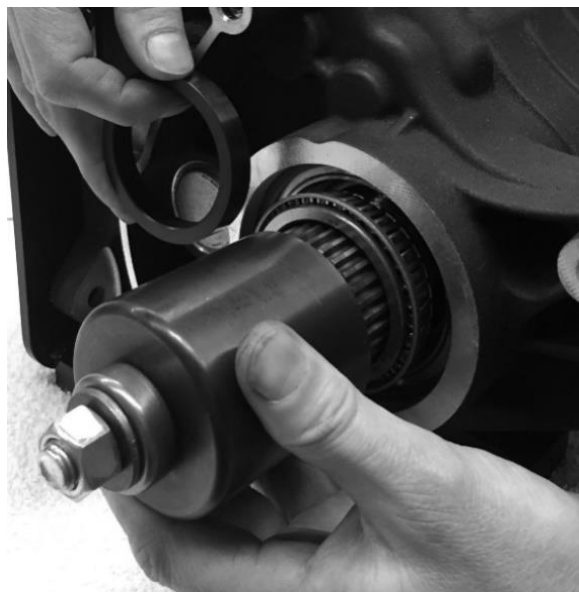
FIGURE 15 | IF USING H-D TOOLING, THE INCLUDED PULLEY SPACER IS NEEDED TO EXTEND THE LENGTH OF THE INSTALLATION CUP
