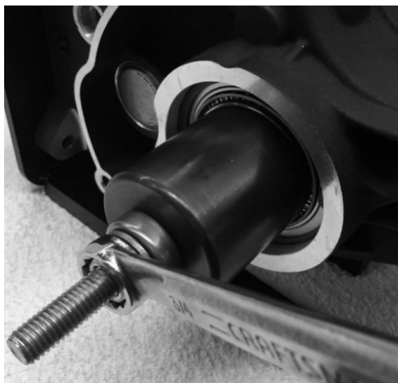
FIGURE 16 | INSTALLING THE MAIN DRIVE GEAR
