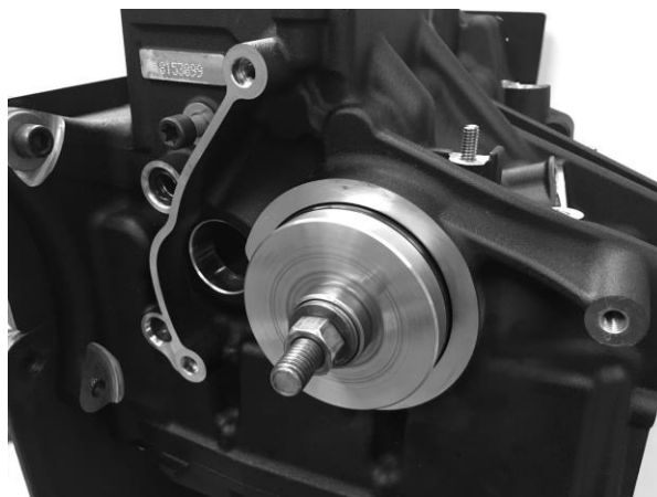
FIGURE 5 | TAPERED BEARING ADAPTER TOOL SETUP, LEFT SIDE VIEW
