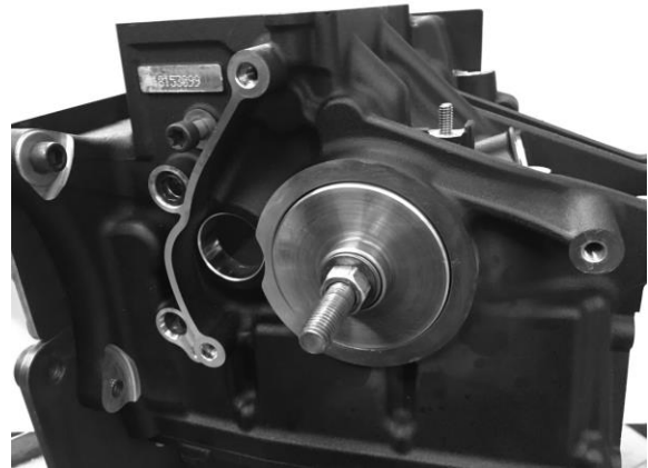
FIGURE 10 | TAPERED BEARING ADAPTER FULLY SEATED IN CASE
