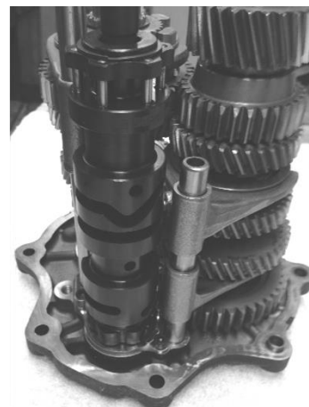
FIGURE 5 | NEW BAKER SHIFT SYSTEM INSTALLED
