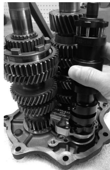
FIGURE 4 | INSTALLING BAKER SHIFT SYSTEM
