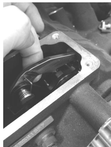
FIGURE 7; PULL PAWL ARM OVER SHIFT DRUM DURING INSTALLATION
