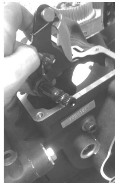
FIGURE 6; INSTALLING NEW SHIFTER PAWL
