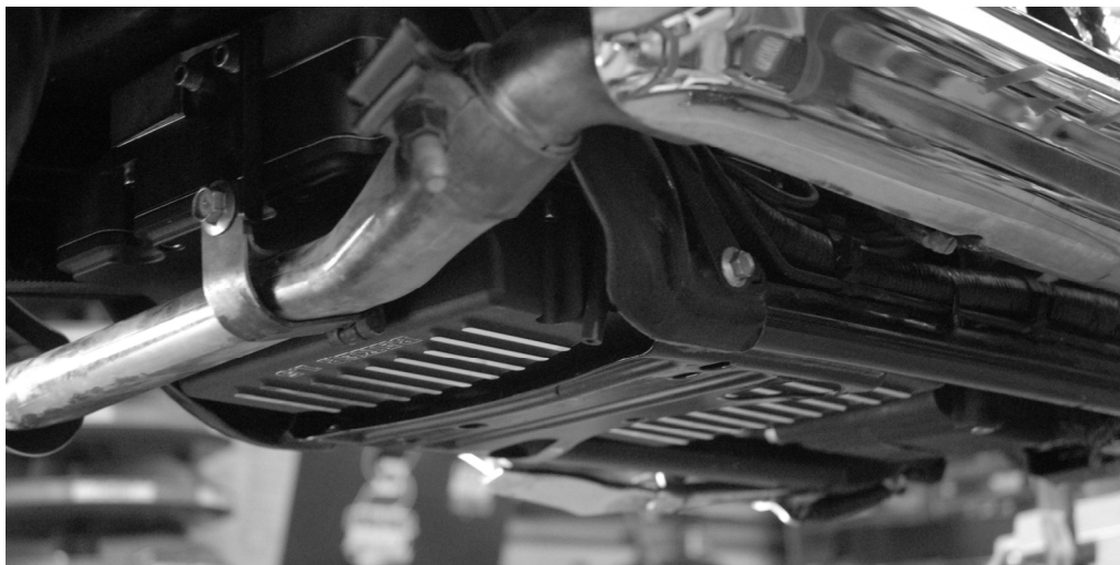
BAKER 1.5 OIL PAN INSTALLED, FIGURE 11
