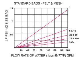
The value obtained in step 3,  $\Delta PB$  is the clean pressure drop caused by the filter bag.
