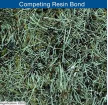
The 50x magnification images of two clean filters demonstrate how the **ECO-RBU** achieves such incredible open area (void space) improvements compared to traditional resin bonded filters.
