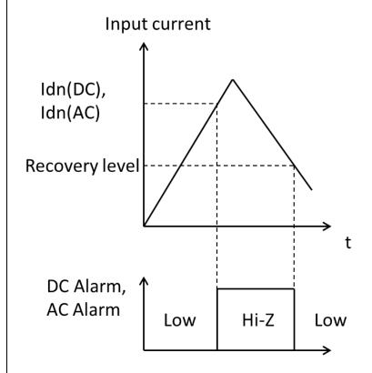
When the residual current exceeds the threshold level (Idn(DC) or Idn(AC)), PIN 4(DC Alarm) or PIN 5(AC Alarm) will change from low level(GND) to high impedance. Each output goes back from high impedance to low level when residual current falls below recovery level.
