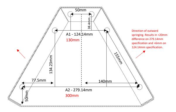
The A1 and A2 measurements need to match the physical product. If these measurements are proving challenging to achieve within a lesser tolerance, perhaps an ellipse hole would overcome the challenge and ensure install is made easier?
