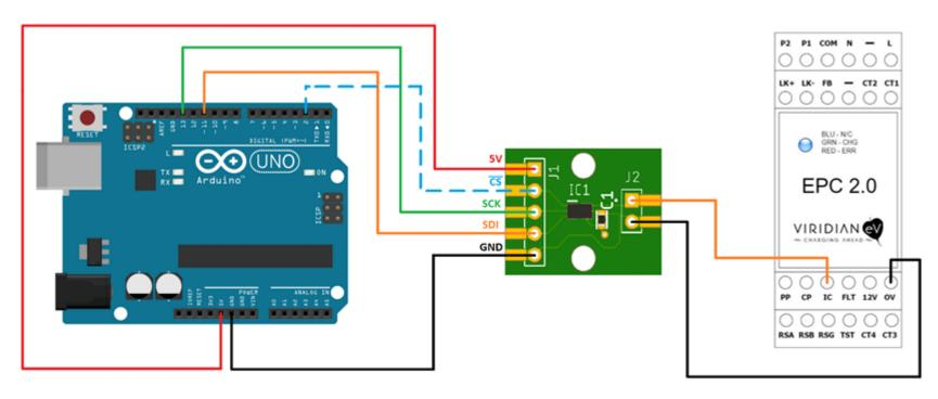
**Note:** The **cs** pin can be connected to any unused GPIO pin.
