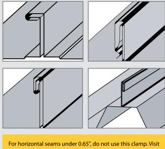
For horizontal seams under 0.65", do not use this clamp. Visit www.S-5.com for more detailed information and proper clamp usage.
