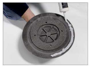
**STEP 6:** Lay cover plate onto base plate, taking care to align it using the indicator marks made in Step 4.
