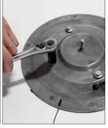
**STEP 8:** Once the cover plate is secured to the base plate, inspect to ensure that water block sealant has squeezed out around the edges of the top disc. Apply more water block around the edge of the disc if necessary.
