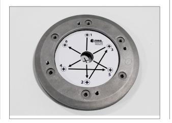
**STEP 4:** Once the base plate is attached to the roof, loose lay the cover plate over the base plate by aligning the bolt holes. Once the bolt holes are properly aligned, mark the cover plate and membrane as shown to help re-align the cover plate for final installation in step 6.
