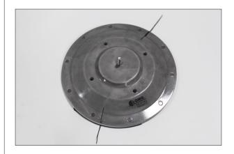
**STEP 5:** Apply a ½-inch wide bead of water block sealant (specified by roof membrane manufacturer, supplied by others) around the edge of the underside of the cover plate.
