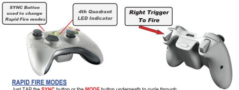
Just TAP the SYNC button or the MODE button underneath to cycle through the modes. At which point the player 4 LED will flash indicating the MODE you are in. The chip will remember the speed mode (no BURST/AKIMBO), even when you turn your controller off or remove the batteries.
