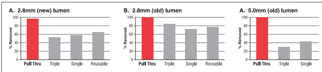
Percent of soil removed (Mean  $\pm$  SD) from the lumen after passage of the lumen-cleaning device.
