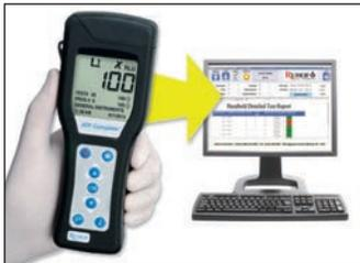
The hand held unit can then be synced to a PC where the reading is down-loaded to an easy-to-use database management software for tracking the results. The software program can be used to run comparison charts and produce color trend analysis graphs and reports.
