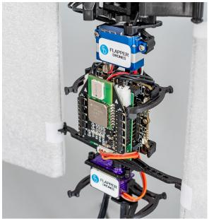
**Figure 1:** On-board electronics stack with integrated pin headers for 1 expansion deck: Pin header location (left) and installation of the LPS deck as an example (right)
