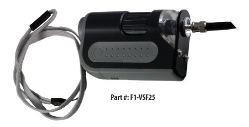
Our fiber inspection scope provides a crystal clear view of both the cladding and core of a ber connector endface to locate defects or contamination. Our standard scope includes a universal 2.5mm adapter that accepts SC, ST or FC connectors in either an APC or UPC configuration.
