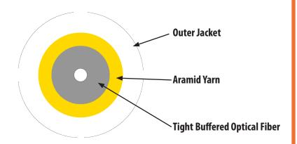
Zeus presents: MDU Drop Fiber: The MDU Drop fiber is composed of 1 fiber Corning ClearCurve® ZBL Indoor / Outdoor Riser cable, terminated with (1) SC/APC or (1) LC/APC Green Connector, and spooled on a 7 inch spool.
