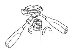
Set the new head, or accessory on the tripod's threaded post, and turn clockwise until it comes to a stop.
