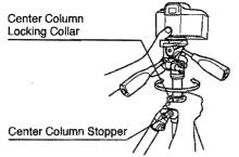
Hold onto the Pan Head with one hand, and loosen the Center Column Locking Collar with the other hand.
