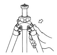
After choosing the desired leg angle, securely push in the Adjustment lock
