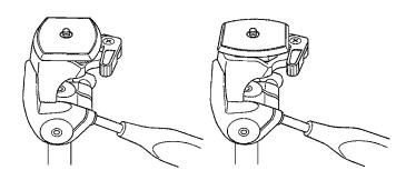
The Quick Release Platform can be attached to the camera body in either directions (along the length, or along the width).
