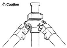
Make sure to re-attach the Base Stopper, in order to prevent the Center Column from falling out.
