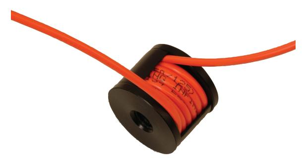
The use of mandrels in multimode insertion loss testing helps to ensure the proper launch condition into the fiber under test. By wrapping the fiber around the correct size mandrel, high order modes are stripped out and low order modes are spread out to achieve the desired launch conditions for testing. Each includes the mandrel and clip for holding the cable firmly in place during testing. Accepts jacket diameters from 1.6mm to 3.0mm and for use both OM1, OM2 cable.
