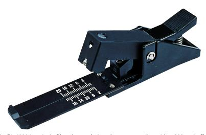
The F1-6000 is a single fiber cleaver designed to accommodate either 900um buffered or 250um coated fiber. The F1-6000 cleaver's quick and easy three-step operation is well suited for mechanical splice and quick termination field connector applications. The leaf spring base is ruled to allow for cleave lengths of 2 to 20mm. The standard carbide blade will perform up to 6000 cleaves before replacement.
