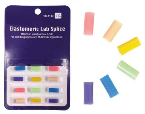
We now offer a new and improved Elastomeric Lab Splice. The splice is ideal for making temporary fiber connections, since it can be disassembled and reused hundreds of times. To install the splice for instrument testing, simply insert a cleaved pigtail from an OTDR or power meter to the cleaved unconnector-ized fiber.
