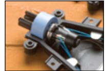
Cable Retention with Bobbin
