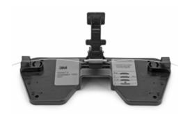
4.9 Pivot the handle of the 3M™ Fibrlok™ Assembly
