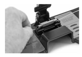
4.6 Gently push the second fiber in small increments straight through the alignment guide into the fiber entry port. As the coating of the second fiber enters the fiber entry port, watch for the bow in the first fiber to increase. This occurs when the end face of the second fiber contacts the first fiber and pushes the first fiber slightly back out of the splice. Continue gently pushing the second fiber until it meets resistance.
