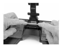
2.4 If using the 3M™ Fibrlok™ Assembly Tool 2501, rotate the toggle arms for the appropriate fiber size.
