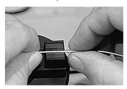
4.2 Grasp the coated fiber about .25 inches (6 mm) from the bare glass and move the fiber end onto the fiber alignment guide on the assembly tool such that the end is resting on the alignment guide outside of the splice.
