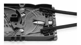
6.4 Place the splice assembly tool close to or on top of the splice tray. Match the orientation of the tool to that of the splice holder or tray whenever possible.
