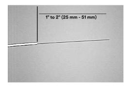
3.3 Clean the bare glass by pulling the fiber through an alcohol soaked lint-free wipe. This will remove any fragments or dirt remaining on the fiber.
