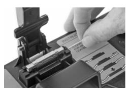
Note: Push fiber <u>straight</u> into fiber alignment guide, <u>NOT AT AN ANGLE</u>.
