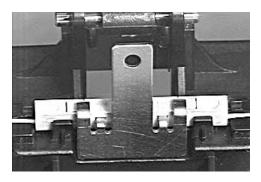
5.3 Slide the bottom of the cap lifter inward until it is in a vertical position, lifting the splice slightly out of the cradle.
