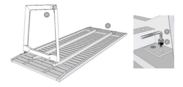
**Step 3**Add the screws as shown in the figure. Repeat Step 2 and 3 for the other leg.
