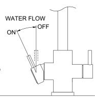
Ceramic disc cartridge diverter valve is auto-off except under conditions of low or unreliable water pressure, sediment in water, lime, salt, iron or other mineral deposits, etc., in which case it must be disengaged manually by the user.
