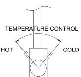
Ceramic disc cartridge mixer valve controls water flow and temperature
