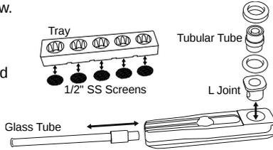
isopropyl alcohol. Push the screens back into place when done. Remove the Glass Tube by sliding it out from the Battery Cover/Mouthpiece then remove the L joint. Clean both with isopropyl alcohol and/or a pipe cleaner.
