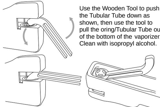
To re-assemble, start by putting the top two o-rings into place beneath the heater. Use the wooden tool to ensure they lay flat. Slide the tray all the way into place, turn the vape over, then push the Tubular Tube into the hole so that the 3 holes in the Tube are on the bottom side of the vaporizer. Push the final o-ring down around the Tubular Tube.
