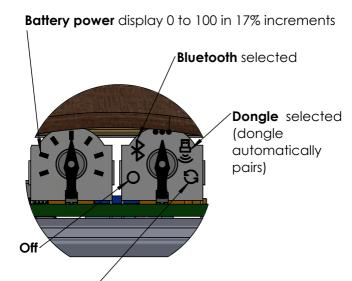
To pair Bluetooth, first, select Bluetooth icon using the connection button. Then press the Bluetooth button. The display points to the pairing icon when pairing mode is entered. When pairing is successful, the indicator points back to the Bluetooth icon.
