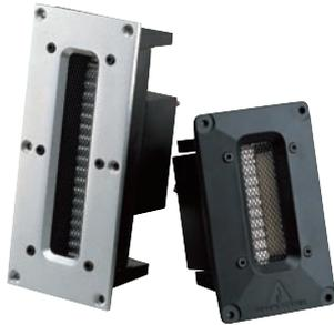
Fundamental physics explains why the ribbon is the perfect type of transducer. Instead of using a cone attached to a voice coil suspended in a magnetic field, a ribbon driver uses a strip of aluminum foil ribbon as a diaphragm. It is suspended between the opposite poles of two magnets. As the signal current passes through the electrically conductive ribbon, it interacts with the magnetic fields. This causes the ribbon to move back and forth, creating sound.
