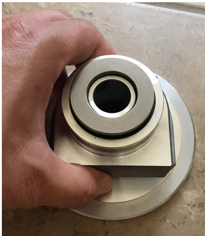
remove the black plastic bearing cover first
