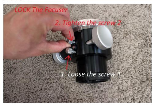
2. Fine-tune the focus for eyepiece. You could adjust adequate focuser friction you would like.
