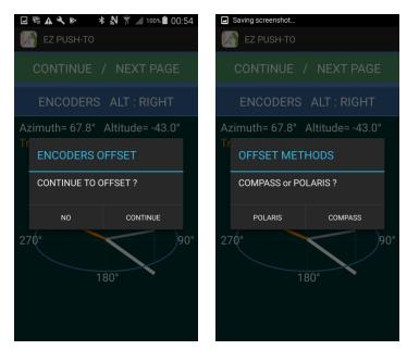
\*After Pre-Offset Encoders, check and confirm az/alt displayed correctly.
