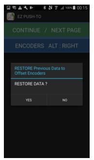
Set the ALT encoder installed at LEFT/RIGHT(default) hand side \*wrong side makes altitude encoder readout reversely.
