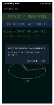
Set the ALT encoder installed at LEFT/RIGHT(default) hand side \*wrong side makes altitude encoder readout reversely.
