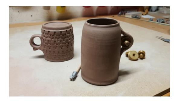
3. An extruded vessel using the **Rélyéf Extruder Hollow Dies** for the Nidec Shimpo EX 115 press.
