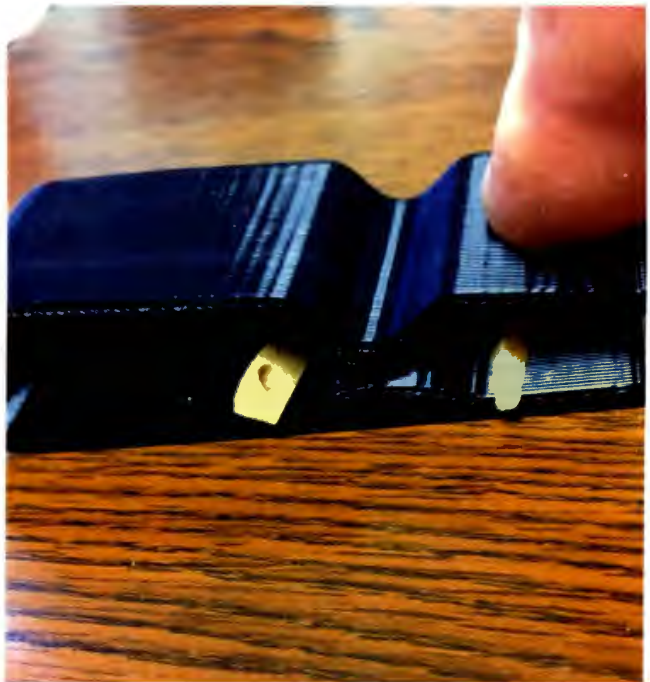
#4- press down as shown to separate cones
