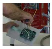
Your new controller was shipped with a Static Bag. Place your old control board in the Static Bag for storage, just in case you need a backup.
