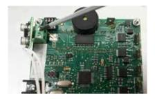
5. Next, remove the Thermocouple Wires. Loosen all of the thermocouple leads and remove the wires from the block.
